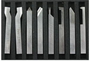
The 8 piece set above includes, turning, facing, finishing, Parting/grooving. boring, internal and external thread cutters. For the very occasional turner of softer materials, this option is close to being completely adequate. Prices range from \$77 for the 8 piece set to \$181.50 for the 12mm set
