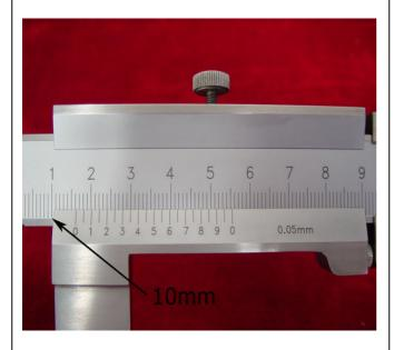
2). Find the millimeter mark on the fixed scale that is just to the left of the 0-mark on the vernier scale. (6mm on the fixed caliper)
