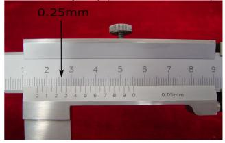
4). To get the correct reading, simply add this found digit to your previous reading. (10mm + 6mm + 0.25mm= 16.25 mm)
