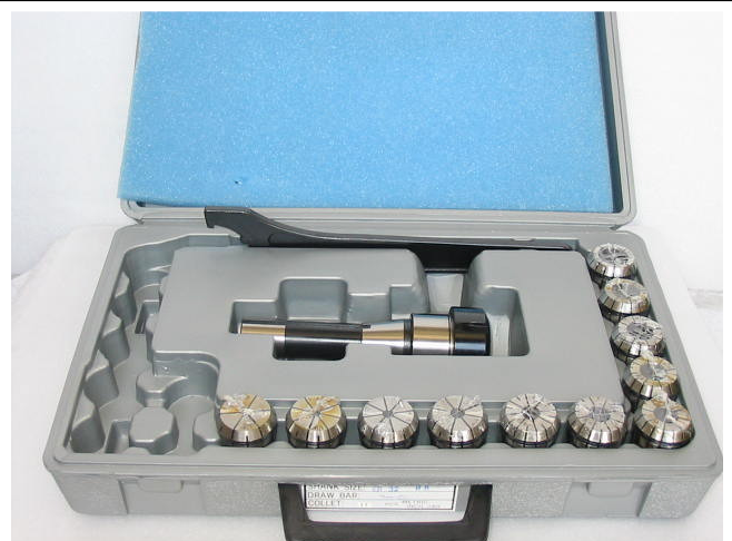
ER Collet Set showing Collet chuck with R8 taper arbor, locking nut, C Spanner and range of collets (Selectable)
