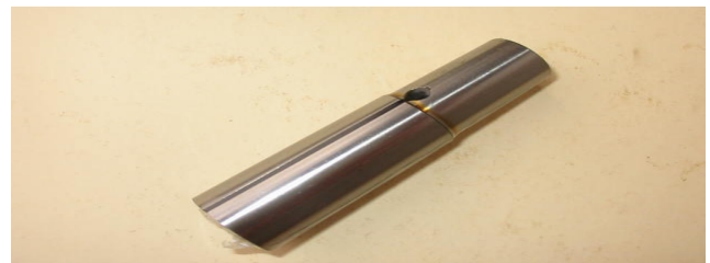
Morse Taper collet for inserting directly into the spindle. No chuck necessary but drawbar is required.
