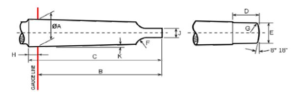
**Brown & Sharpe** Like the Morse, these have a series of sizes, from 1 to 18, with 7, 9 and 11 being the most common. Actual taper on these is within a close range of .500" per foot.
